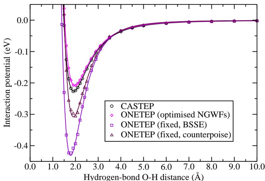
**Fig. 10** Interaction potentials (negated binding energies) for a hydrogen-bonded water dimer.
